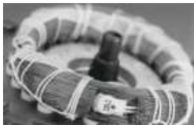
Fig. 46 Thermal switch incorporated in windings
