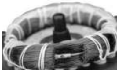
Fig. 44 PTC sensor incorporated in windings
